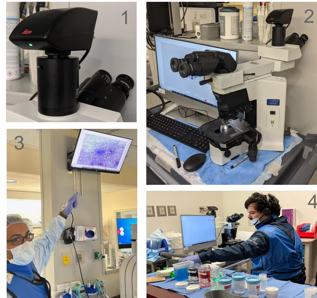
Figure 1: Workflow setup within the bronchoscopy suite. (1) refers to the Leica Flexacam C3, connected to (2) the Olympus BX43 Microscope. Live images from the microscope are broadcasted (3) for the interventional pulmonologist. (4) shows the overall mobile station that the cytotechnologist uses to communicate with the remote pathologist at another institution.
